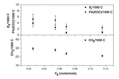
Figure 2. Course of methyl groups (CH $_3$ /1000C), butyl short chain branches ( $B_4$ /1000C) and end of chain contributions caused by transfer to propionic aldehyde (PA(EOC)1000C) as a function of styrene co-polymer mole fraction  $F_5$ .
