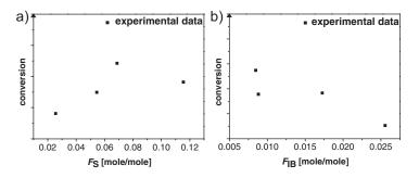
Figure 1. a: Course of conversion as a function of styrene mole fraction  $F_S$  in co-polymer. b: Course of conversion as a function of isobutene mole fraction  $F_{IB}$  in co-polymer.
