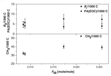
**Figure 3.** Course of methyl groups ( $CH_3/1000C$ ), butyl short chain branches ( $B_4/1000C$ ) and end of chain contributions caused by transfer to propionic aldehyde (PA(EOC)1000C) as a function of isobutene co-polymer mole fraction  $F_{IB}$ .
